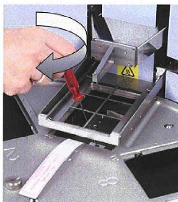
Figure 3-27. Refitting the transport lock of the heating block (B)
